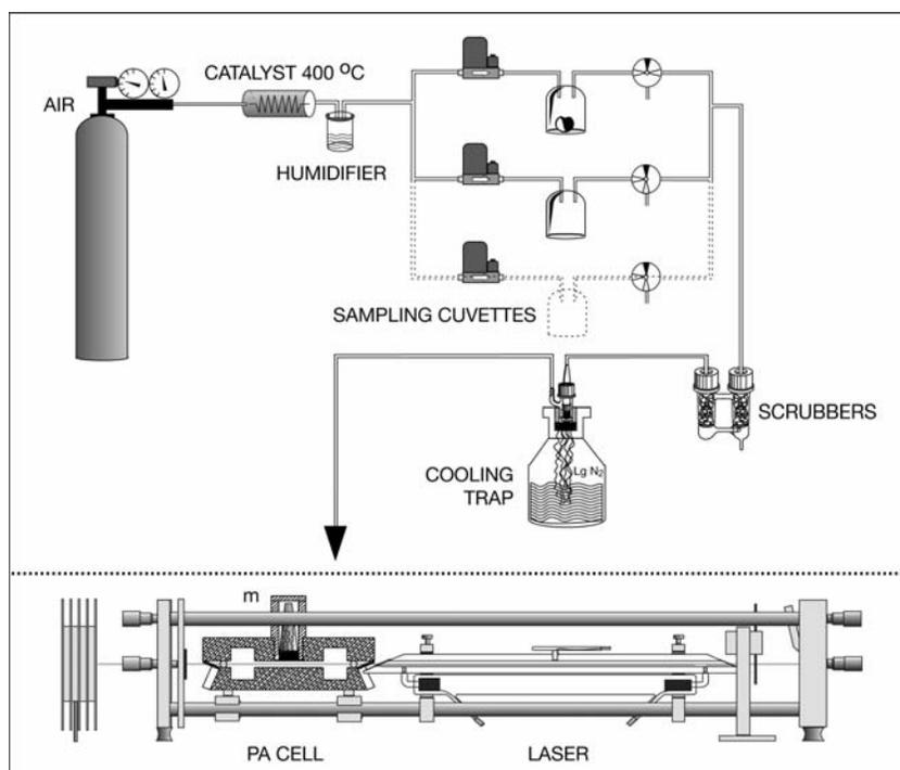
Figure 2. The ethylene detection set-up. A) gas flow system. B) laser-based ethylene detector consisting of a photoacoustic (PA) cell and a CO<sub>2</sub> laser. Ethylene released by the biological samples (plated fungi or infected fruits) is transported to the PA cell where it absorbs the laser radiation and gives rise to an acoustic wave. The amplitude of this wave is measured with a sensitive microphone (m) and is directly proportional with the ethylene concentration.
